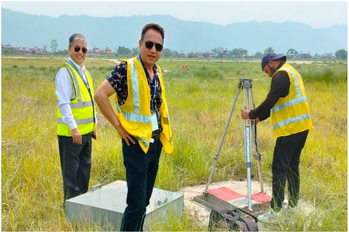
Instrument orientation for Static DGPS observation at control point established by Pokhara International Airport
