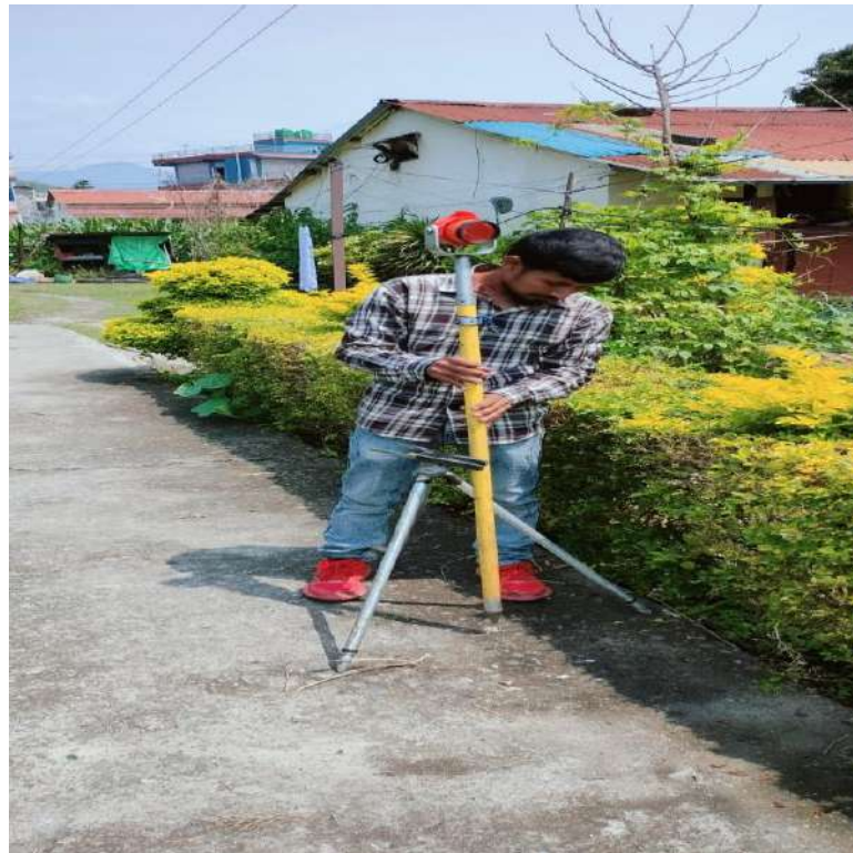
Back sight target orientation for Total Station Survey
