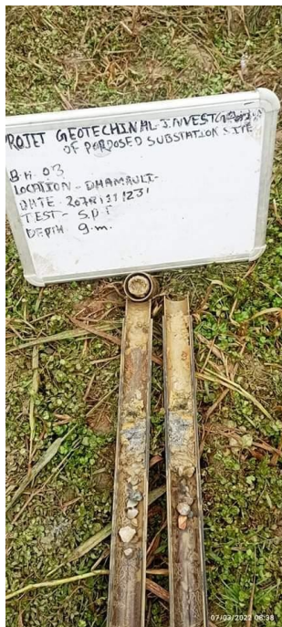
Soil Sample in Split Spoon Sampler of New Borehole 3 of Damauli SS; Depth 9 m
