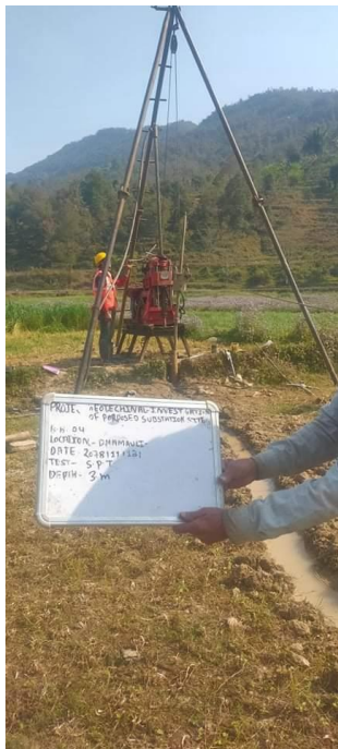
Conduction of Standard Penetration Test at New Borehole 4 of Damauli SS; Depth 3 m
