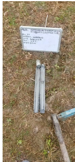
Soil Sample in Split Spoon Sampler of New Borehole 4 of Damauli SS; Depth 7.5 m
