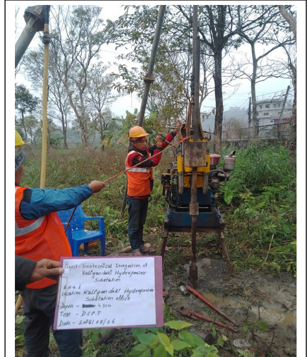
Conduction of Dynamic Cone Penetration Test at Depth 4.5 m
