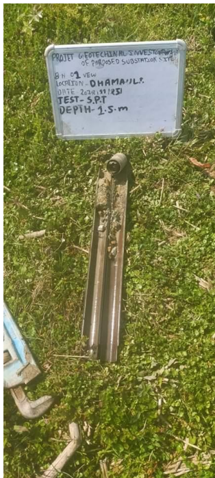
Soil Sample in Split Spoon Sampler of New Borehole 1 of Damauli SS; Depth 1.5 m
