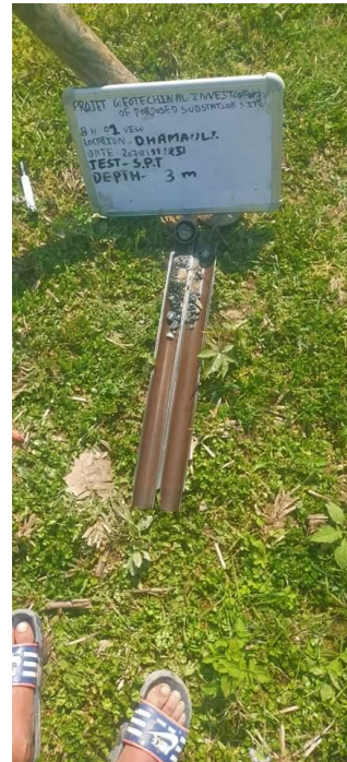
Soil Sample in Split Spoon Sampler of New Borehole 1 of Damauli SS; Depth 3 m
